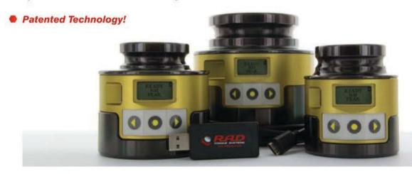
Uses RAD Torque's transducer technology combined with custom sockets to measure the torque applied to the bolt during a torque cycle. By innovative design, the Smart Socket is no larger than a standard socket. It's compact size and innovative technology makes the Smart Socket a perfect audit tool for inspecting bolted joints and can function as a master calibration for various torque tools.
